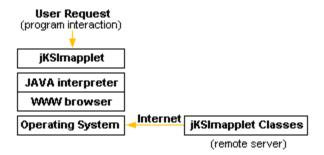
Figure 32. jKSImapplet Execution Structure diagram.
