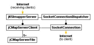
Figure 34. jKSImapper Server Structure diagram.
